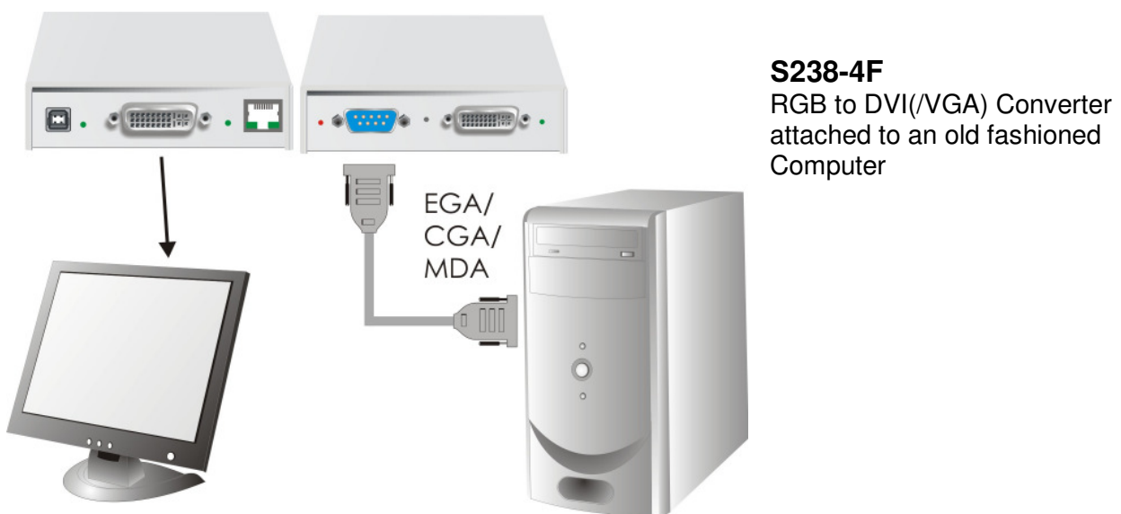
Figure 21 RGB to DVI(/VGA) Converter with optional EGA/CGA support, attached to an old fashioned Computer
